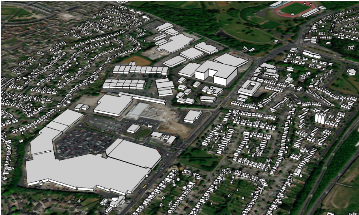
Figure 6.1: CFD Model of the Baseline Scenario
